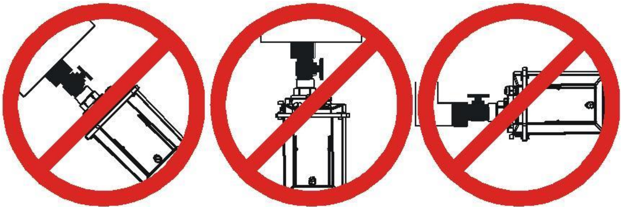
Figure 2-4: Do Not Install the Hydran M2-X at an Angle, Vertically or Using an Elbow
