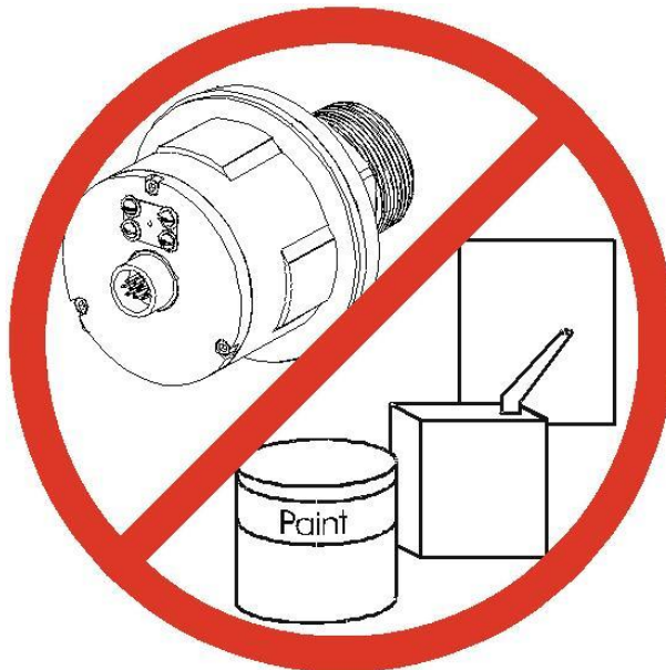
Figure 2-8: Do Not Paint the Sensor or Clean It with Any Solvent
