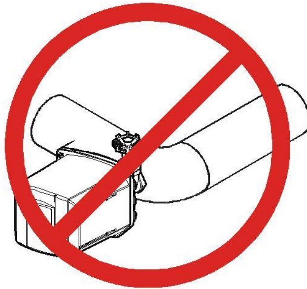
Figure 2-5: Do Not Install the Hydran M2-X on an Elbow or a Fitting Box
