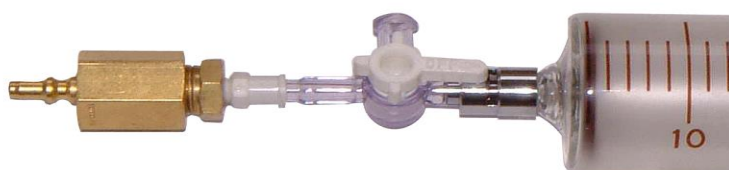
Figure 7-28: Male part of the quick-connector valve attached to the syringe
