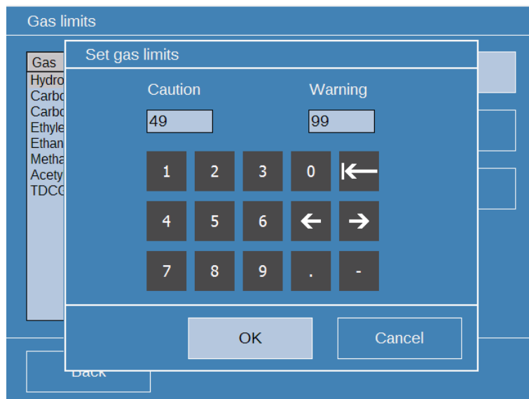
Figure 7-55: Setup > Gas Limits > Edit - values - keypad - new
