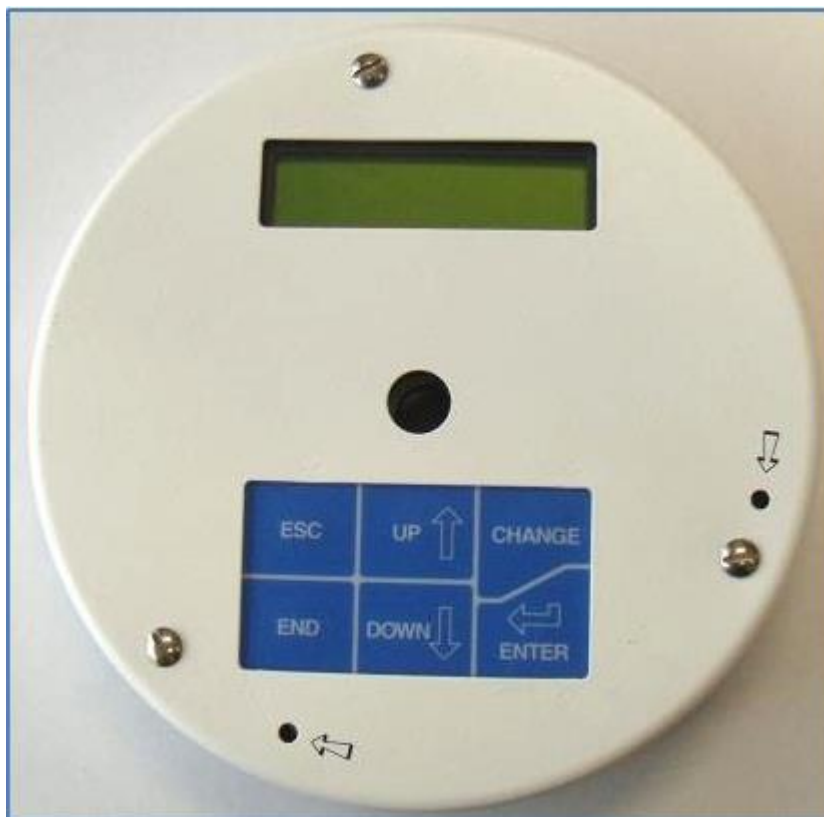
Figure 5-1: Hydran 201Ti's User Interface
