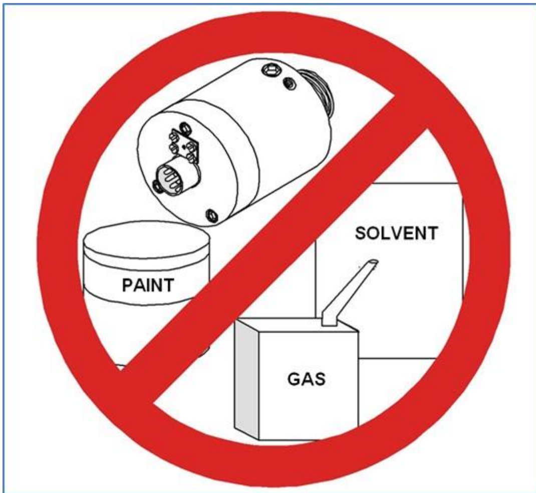
Figure 6-3: Do not paint the Sensor or do not clean it with any solvent
