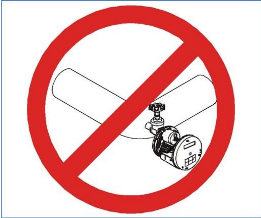
Figure 6-6: Do Not Install the H201Ti on an Elbow
