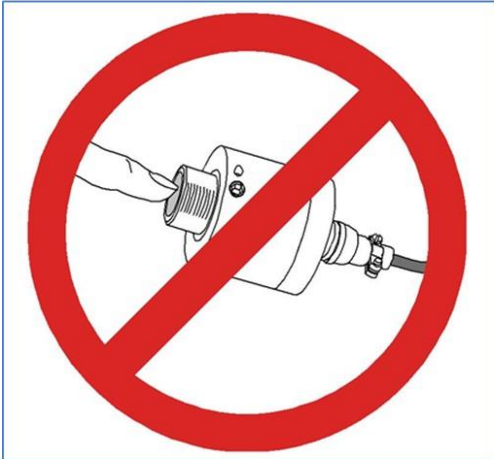
Figure 6-2: Do Not Touch the Membrane
